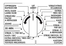
With the programme knob position WOOL/SILK (WOL/ZIJDE), the desired programme can be selected with the WOOL (WOL) or SILK (ZIJDE) buttons. If no button is pressed, the WOOL (WOL) programme is automatically set.
